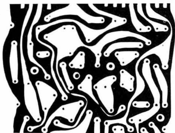
Fig 1. Example of pcb produced from pen and ink drawings. The master is normally drawn two or three times full scale and then reduced by photographic processes. Printed circuits drawn directly on to the copper laminate with an etch-resist ink pen are usually in this style
